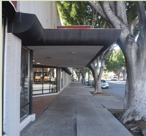
Wider walk zones of at least 6 feet are appropriate for commercial retail areas
