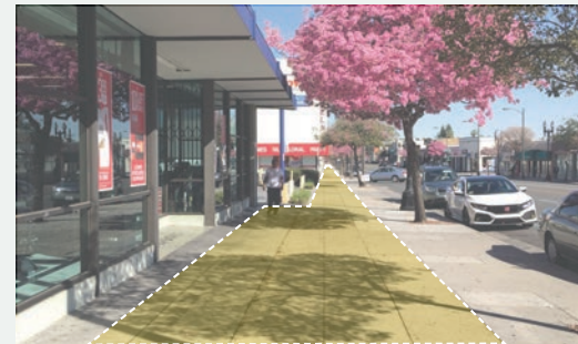
Walk zones may extend into frontage zones if desired by the property owner
