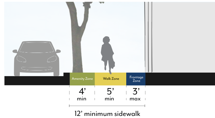
Figure 5.1-6: Sidewalks - Green Street (Mid-City & South Green)
