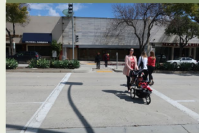
Signalized crossings in-between major intersections can improve pedestrian safety and facilitate connectivity by breaking up long blocks
